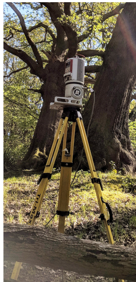
NCEO-UCL's Riegl VZ-400 terrestrial laser scanner (TLS). The instrument sends out hundreds of thousands of laser pulses per second to make an extremely detailed 3D picture of these 200-year-old oaks in Hampstead Heath. These measurements are used to help estimate the atmospheric CO 2 absorbed by urban trees during photosynthesis. Credit: M. Disney and P. Wilkes, NCEO-UCL.
